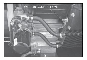
Figure 32. Wire 18 Connection 10-20 kW Units
